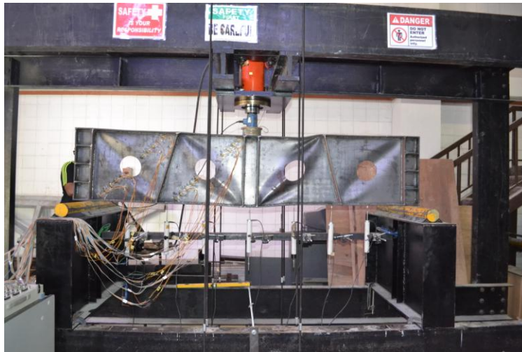
Figure 7. Typical deformation of girder at failure.
