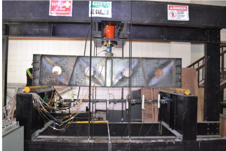
Figure 6. Typical deformation of webs at critical buckling load.
