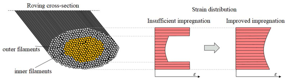
Fig. 1. Stress distribution due to poor impregnation according to Lepenies (2007).
