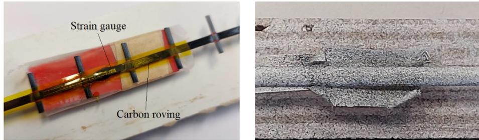
Fig. 3. Applied strain gauge and gray-scale pattern for the DIC.
