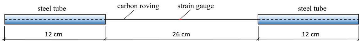
Fig. 2. Specimen geometry.
