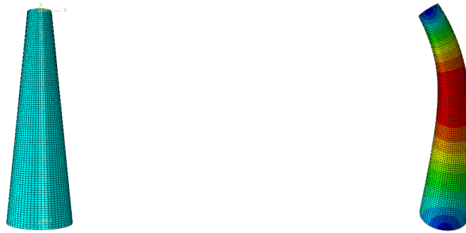
Fig. 5. Model geometry with the meshing and first buckling mode of a tapered annular cylindrical column.
