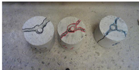
Figure 5. Failure pattern of specimens depending on the fiber volume content 0%, 4%, and 8%.
