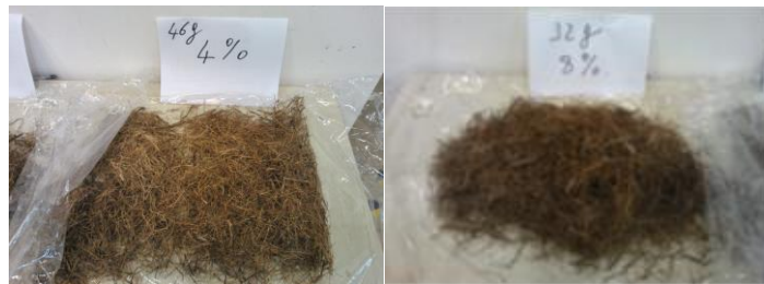
Figure 2. Weight of agave fiber for samples 4% and 8%, in volume content, respectively.
