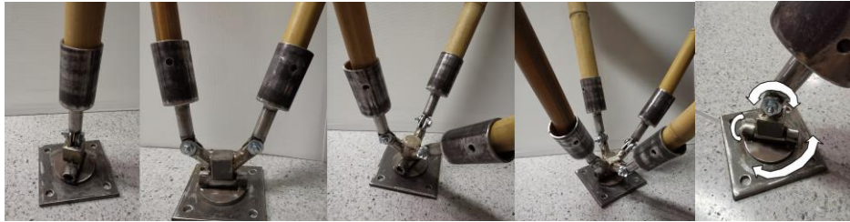
Figure 7. (Four Left) Designed male and female connectors are demonstrated when they are assembled together, (Right) Multiple axis of connector allows flexibility of structural member's movement.
