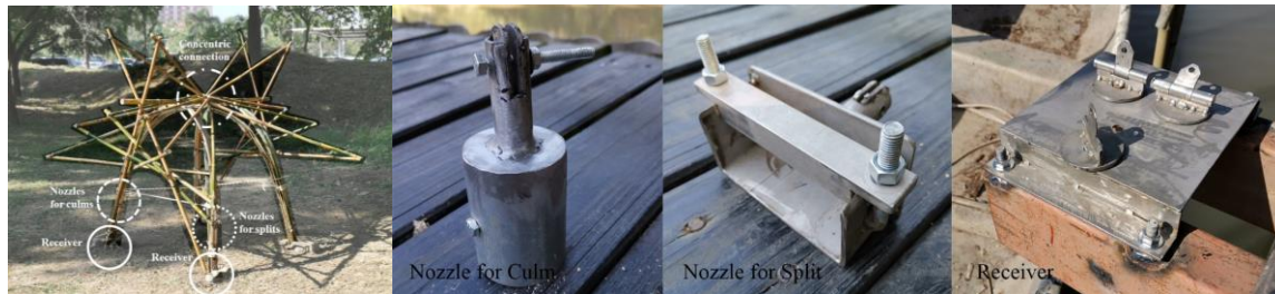
Figure 4. (Left) The model of structure prototype to explore connections, (Three on Right) Three experiment connectors to be installed on prototype. They are nozzles and receiver at base joints.
