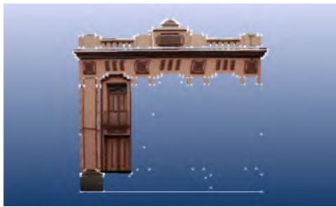
Figure 4. Model surface generation through referenced points (Ochoa 2003).
