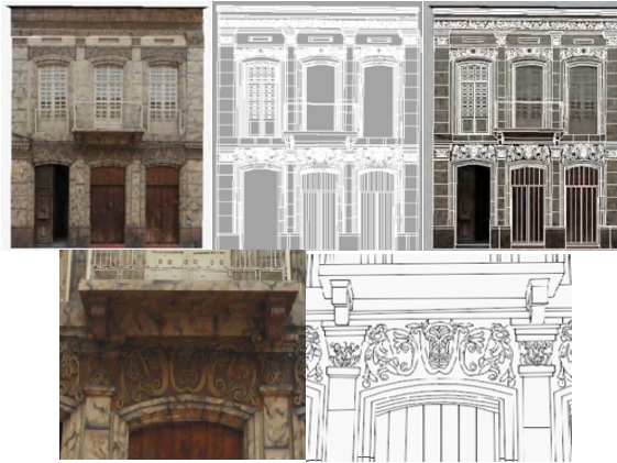
Figure 8. Orthophoto, digitalization and detail of building facade located at Benigno Malo Street 6-34 in Cuenca, Ecuador (Universidad del Azuay 2003).
